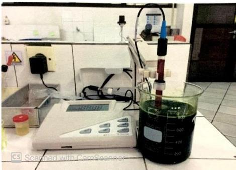
**Gambar 2b - Oxidation Reduction Parameter**
