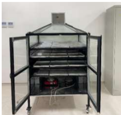
Gambar 1. Rangkaian alat electric tunnel dryer
